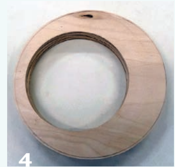
4 The 6" ring has a 4" hole offset by 1/2".
