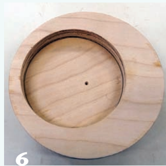
5 The completed chuck body has a centered tenon on the back side and an offset recess on the front side.
