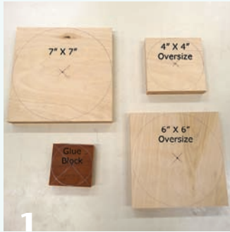
1 You will need three plywood squares for the body of the chuck and a piece of hardwood for the tenon.
