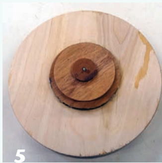
5 The completed chuck body has a centered tenon on the back side and an offset recess on the front side.
