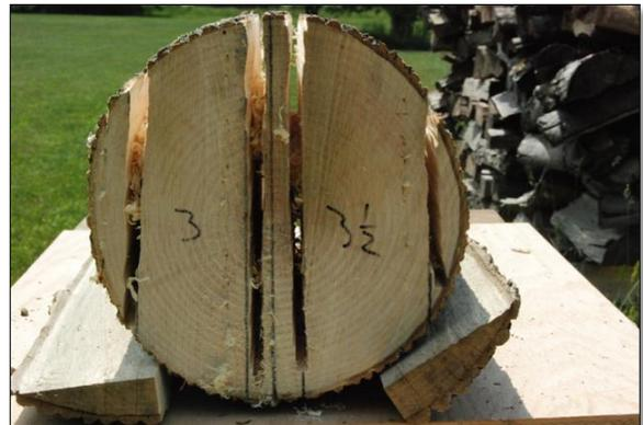
*Figure 8: Don't cut all the way through the log when making the initial cuts. The log will be more stable and safer done this way. Once all the cuts are made, you can go back and finish the cuts starting with the two outside cuts.*
