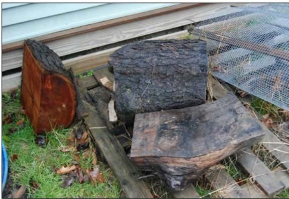
*Photo 1: Blanks are best kept as large as possible unless used quickly.*
