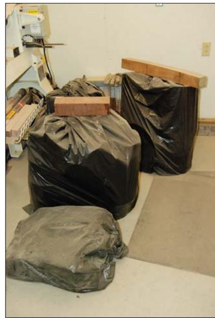
*Photo 5: Storing the blanks in a large plastic bag is one way to prevent checking.*
