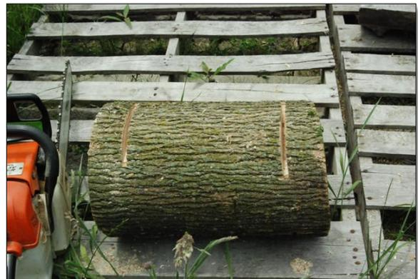
Figure 2 shows the log laid out, ready to be cut to length. I cut the section out in the middle of the log in order to eliminate any cracking that was present on the ends. You will have to keep reducing the length until all the cracks are gone, even if it means working with a smaller blank. There is no point in trying to turn cracked wood! Try to get as square a cut as possible when cutting to length.
